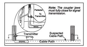
Connect the Dyna-Coupler to the Transmitter front panel jack using the coupler cable.
